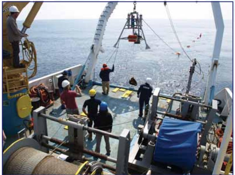
Oceanlab's BRIL being deployed in the Santa Maria di Leuca Coral field in April 2010 from the R/V *Universitatis*. The mooring line carrying the floats is already in the water behind the vessel, and the ballast and bait are visible hanging below the lander frame.
