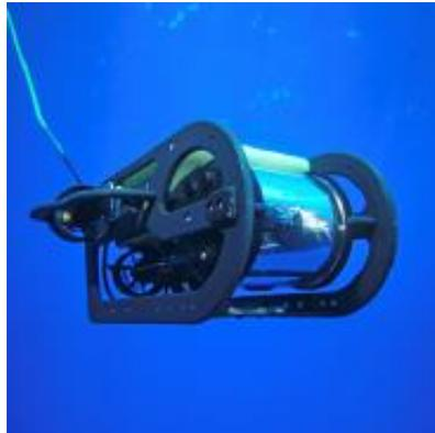
The DOP/UAz ROV: a SeaBotix LBV300S-6, rated to 300m & equipped with 2 cameras: one colour
